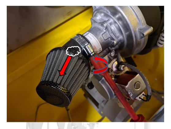
Unscrew and remove air filter from whole burner, then use compressed air to clean the surfaces from the inside. After these steps, screw it back.
