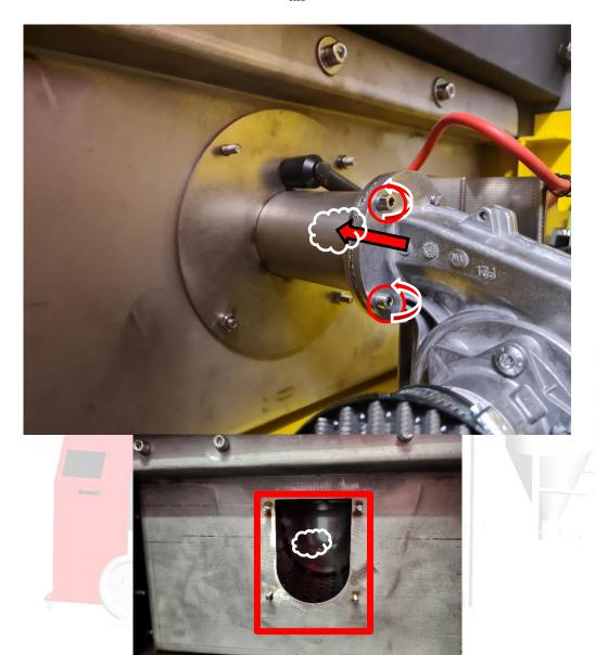
After cleaning the burner and burner grille, assemble the components. After these activities, check the gas system for tightness and the correct operation of the flame and ignition control system!
