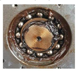
**Step 3.** Start the cleaning process by getting rid of the old grease. In this case, use the old cloth or brush.
