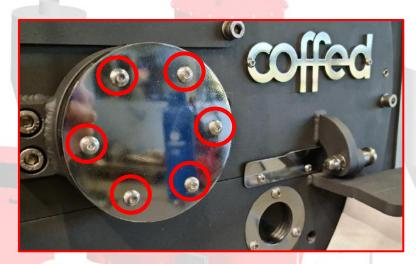
**Step 2.** Unscrew and then remove the securing screw:
