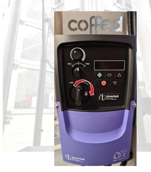
**3.** With the device turned on, the knob marked in the figure below should be turned to the left or right (these positions contain the same flow - "reverse" or "forward").
